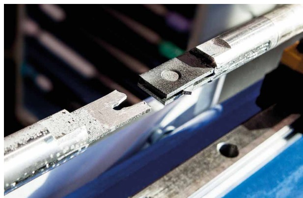
2 Hybrid joint after tensile test at the split Hopkinson tension bar at ten meters per second.
