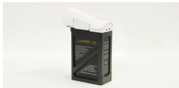
2 Typical lithium ion battery (with a mass of approximately 700 grams) as it is used in a drone.
