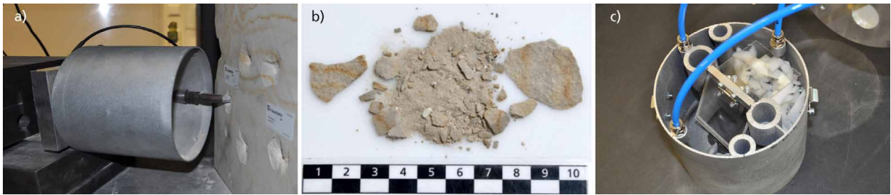
2 Performance test with D-MEN: a) material extraction at a slanted angle in a test chamber, b) extracted material, c) collected material.
