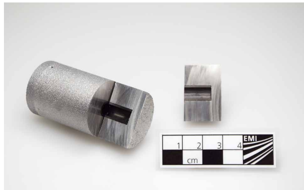
2 Multi-material structure: 3D-printed metallic structure with integrated, conventionally produced composite (split sectional view).
